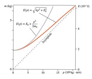
Fig. 1. Relationship between mass/energy and momentum (red line). For large values of the momentum the curve approaches the asymptote (dashed line), for small values the classical quadratic relation (grey line).
