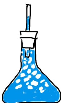
Fig. 1. The amount of entropy that is to be measured is transferred to the ice-water mixture. The amount of the melting ice is a measure of the entropy that has been supplied.
