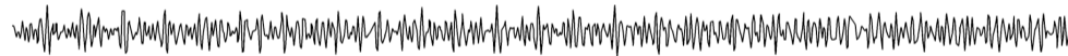
Fig. 2. White light: Field strength at a given point as a function of time
