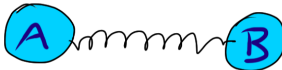
Fig. 1. The spring is under tensional stress. The momentum of A increases, that of B decreases (the “negative momentum” of B increases).
