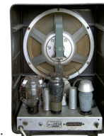
Technical: regenerative audion receiver Historical: notorious propaganda machine
