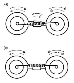
Fig. 3. (a) Demonstration of nondissipative spin-orbit coupling. The sense of rotation of both wheels is identical and opposite to that of the system as a whole. Both senses of rotation oscillate in sign. (b) Demonstration of nondissipative spin-spin coupling. The wheels rotate back and forth in opposite directions. The system as a whole remains at rest.
