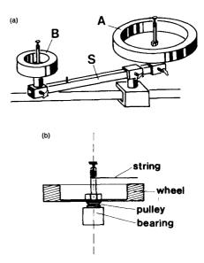
Fig. 1. (a) Two flywheels A and B are attached to a horizontal bar S. Each flywheel is free to rotate about its own vertical axis on the bar and the whole arrangement can rotate about a vertical axis through its center of mass. (b) Detailed illustration of the construction of each flywheel.
