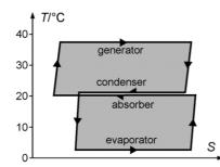
**Figure 5.** *T*–*S* diagram of the absorption refrigerator.
