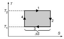
Figure 3. *T*–*S* diagram of the Carnot cycle.
