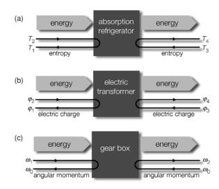
Figure 6. Flow diagrams of (a) absorption refrigerator, (b) electric transformer and (c) gear box.
