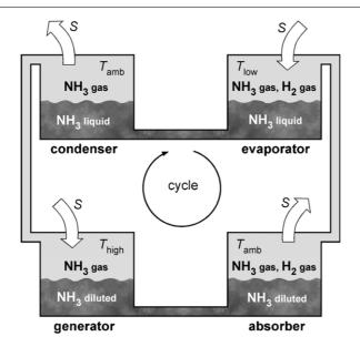
Figure 4. Schematic arrangement of the absorption refrigerator.
